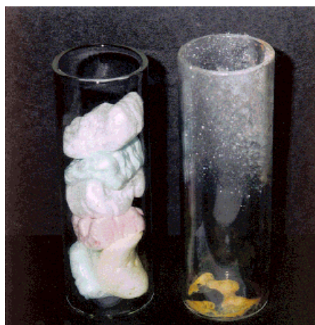
Figure 1. Polystyrene packing material before (left) and after reaction (right) under the standard conditions (170 °C, 16 h; partial pressures: 275 kPa NO, 690 kPa O 2 , 3170 kPa N 2 ). Part of the product mixture can be seen as a sublimate on the liner walls. No unchanged polymer remained.
